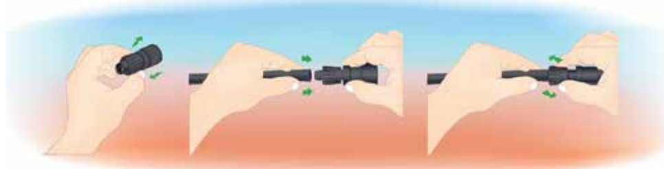
1. Twist collar clockwise toward center of fitting
